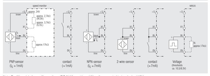
Note: For IK-models the auxiliary voltage (DC 24 V) must be additionally connected to terminals  $\pm U/0V$
